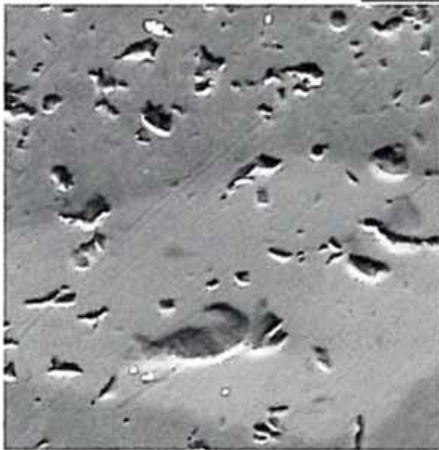
SEM image showing a cross-section of a crack in the ceramic specimen healed with Denseo Fairy.
